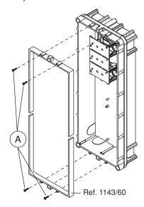
Screws A (3.5 x 16mm) are provided with the spacer.
