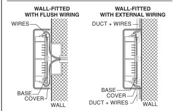
The special decoder presents four holes for wall fastening by means of 6mm diameter bolts (not provided). The decoder can be wall fitted with the wires either flush or not.
