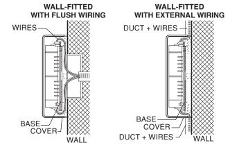
All terminal boards can be removed to facilitate maintenance operations. Wire separators are provided.
