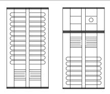
725 panel with aluminium front plate is modular. Various door phone and video door phone configurations can be made by arranging panels and camera units where relevant to obtain the required capacity.
