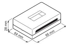
The Ref. 1074/54 distributor is used to share out the VOP video signal from the column to four video door phones.
