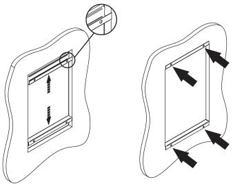
• Fix the box to the wall using 2.9 x 32mm screws.
