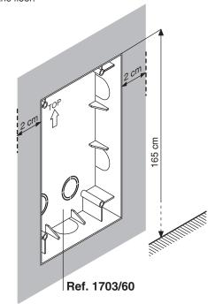
• Fit the frame inside the box and adjust correct perpendicularity.
