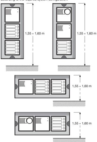
In any case, consider the height shown in the figure for fastening the camera for correct installation of complex arrangement with several modules. The height refers to the door unit in door phone systems.
