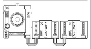
The extension module can be used to add 16 user buttons to the door unit.
