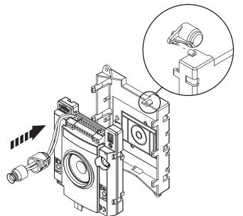
Move the spacer as shown in the following figures to fit the door units:
