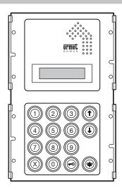
The Ref. 1072/14 calling module corresponds to 2 K-Steel modules and is provided with back-lit 16x2 character display, built-in door unit and back-lit buttons. Flush-mounting boxes or cases with hood and respective frame are required for installation (see "Installation" section).
