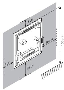
• Fasten the bracket to the wall using the screws and bolts provided or alternatively using a flush mounting box 503 and specific holes.
