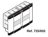
For installation, join the embedding box of the TV camera unit with the push button panel embedding box by means of the white wirespacers (supplied with the TV camera unit). In case of coupling of 2 or more push button panels, couple the embedding boxes by means of the proper black wire-spacers supplied with the push button panels on 2 rows not arranged for loudspeaking unit
