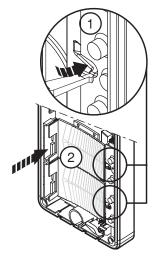
• Insert door unit and handset on base of casing.
