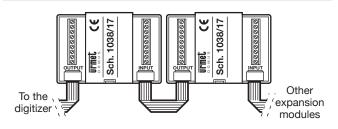
The extension module can be used to add 16 user buttons to the
