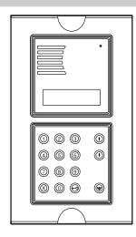
The Ref. 1072/13 calling module corresponds to 2 Sinthesi modules and is provided with back-lit 16x2 character display, built-in door unit and back-lit buttons. Flush-mounting boxes or cases with hood and respective module holders and accessories are required for installation (see "Installation" section).
