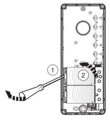
Fasten the casing base on a flat wall, at the height shown in the figure, using the screws (A) and wall plugs (B) provided or on a box Mod. 503.
