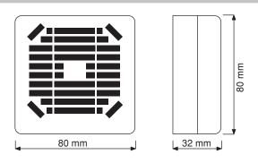
The two-tone supplementary ringer Ref. 1072/59 can only be used with door phone or video door phone with the terminals (or wires) S+ and S- or with the switchboards Ref. 1072/42. The ringer power must be self-standing (by means of 9V battery 6AM6-6LF22) because it cannot be powered by the apartment station.
