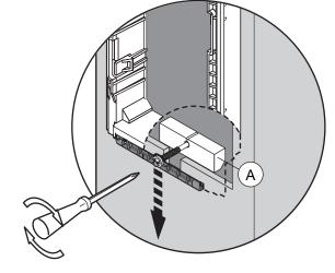
Fasten the modules to the frame, make the connections and tighten the push-button panel using the smaller block, the special screw and spring.
