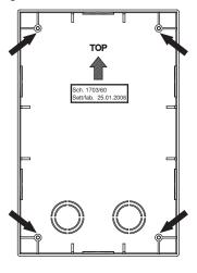
Fasten the adapter brackets of the box with the 3.5 x 9.5mm screws.
