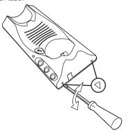
The door phone can be fitted on the wall using the different holes on the base and the special plugs and screws provided with each set.
