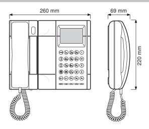
The door phone switchboard Ref. 1072/42 can exclusively be used in Bibus II ed. systems for:
