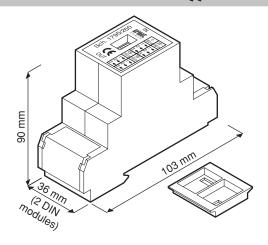
The video signal regenerator Ref. 1795/250 must be used in extended differential video systems (VDE) or Video Over Power (VOP) systems in the event of insufficient video compensation regulation on the VDE brackets or VOP power unit.
