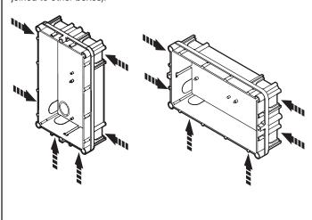
• Fit the flush mounting box in line with the wall: it must not project.
