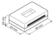
The video distributor Ref. 1795/40 shares out the differential video signal from the main cameras on several riser columns (up to four).
