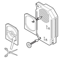
Assemble the panel and camera unit where relevant as shown in the following figure.
