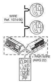
System with several video door phone columns, main video door unit and in-out connection (each column is connected to a secondary electrical door unit)
