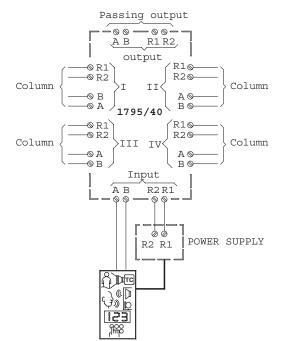
Important: Never fit the video terminal resistors  $82\Omega$  1/4W.
