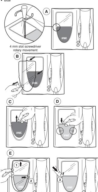
Other media, such as photographs or wall paper, can be used to customise the video door phone instead of the Ref. 1702/50 kit. In this case, use one of the frames provided as a template to trace the exact installation profile.
