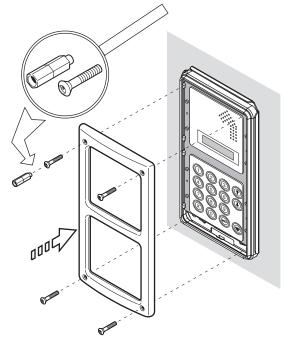
The tool must only be used manually, and not fitted on electrical screwdrivers, to prevent damaging the screws and/or the tool.
