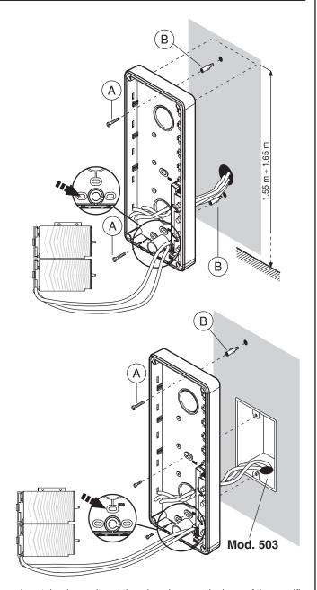
Insert the door unit and the microphone on the base of the specific housing.
