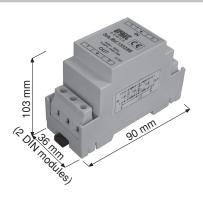
This is a two-cell,high-attenuation,one-phase filter for frequencies >0.1 MHz active on common and differential mode interference. The device is intended to prevent the propagation of external radiofrequency interference on the power mains which could cause faults in the electrical and electronic devices connected to the mains. Install a power line protection device 230V 4000VA Ref. 1332/85 upstream to the power filter to ensure better system operation.
