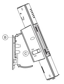
Press lever C and reverse the sequence to remove the monitor.
