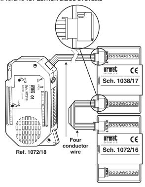
**N.B.**: the buttons associated to the expansion modules will not send the call if the wire is not inserted correctly.
