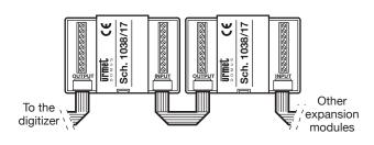
The extension module can be used to add 16 user buttons to the door unit.
