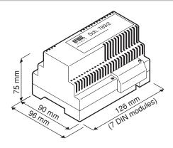
The power unit Ref. 789/2 is required to power the main camera and the video signal Ref. 1795/40 distributor in systems with several column.
