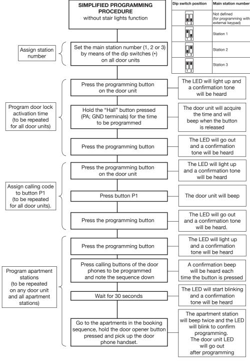
(\*) All data will be lost if the dip switches are moved also after ending the programming procedure.
