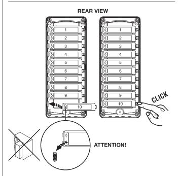
Fit the support with the transparent cover starting from the top downwards.
