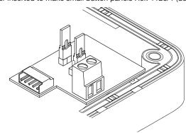
Jumper not inserted to make large button panels Ref. 1128/2.
