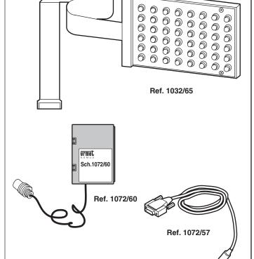
The programming kit consists of the following devices: programming keyboard Ref. 1032/65 Ref. 1072/60 programming adapter N. 1 N. 1 Bibus-PC programming wire Ref. 1072/57
