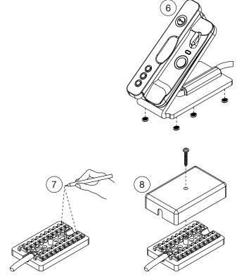
Note the references to the connections on the label of the wiring junction box.
