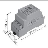
This is a voltage surge varistor power line protection device. The device immediately trips to limit amplitude and preserve the devices installed downstream to the device in the presence of voltage surges generated by atmospheric events. Install a power line filter 230V 4000VA Ref. 1332/86 downstream to the power protection device to ensure better system operation.
