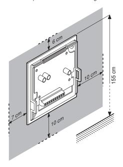
• Fasten the bracket to the wall using the screws and bolts provided or alternatively using a flush mounting box 503 and specific holes.
