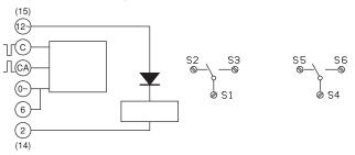
N-1 relays Ref. 788/52 must be used in the system, where N is the number of video door phone units to be connected to the video door phone column.
