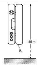
To remove the cover of the door phone, insert the tip of a screwdriver in the area indicated and apply pressure. Extract the cover rotating this on the upper tabs.
