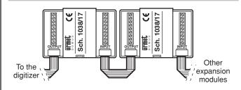
The extension module can be used to add 16 user buttons to the door unit.
