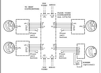
If the 1074/55 device is used instead of the 1074/54, connect the cables of the video signal to the 1074/55 device as connected on the 1074/54. The audio signal cables can be connected to the L1 L2 dedicated connectors as indicated above or leaving the electrical connection set up when using the 1074/54.
