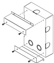
• Break into the plasterboard wall as shown the drawing below.
