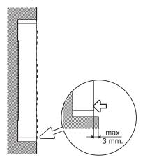
The wall surface must be flat. Maximum permitted tolerance = 1.5 mm.
