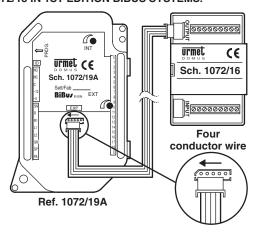
**N.B.**: The buttons associated to the expansion modules will not send the call if the wire is not inserted correctly.
