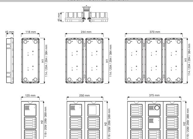
H1= 114, 204, 294, 384 indicates flush mounting height and H2= 119, 209, 299, 389 indicates to total height relative to 1, 2, 3 and 4 module versions.
