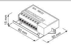
The Ref. 788/22 can be used to repeat calls to a door phone with terminals for connecting a supplementary ringer (S+, S-).
