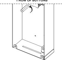
Insert the door unit in the box and fix it by means of the screws 2.9 x 38mm and 3.5 x 8mm included.
