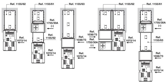
(\*) A colour camera Ref. 1755/45 can be fitted as an alternative.
