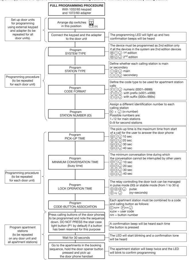
(\*) All data will be lost if the dip switches are moved also after ending the programming procedure.
