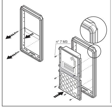
6. Fasten the module holder frame to the flush mounting boxes by means of the specific hinged attachment.
