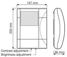
The video module can be installed to the wall by means of a bracket with connector and terminal board.
