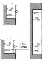
The wall surface on which the front rests must be as smooth as possible (max. tolerance 1.5 mm).
