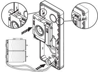
• Connect the wires (it is advisable to have the protrude from the wall by approximately 50mm).
