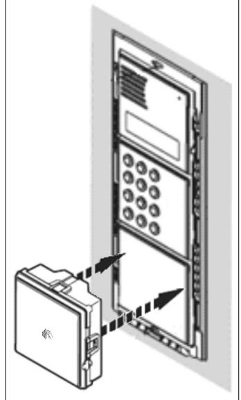
2. Plug module to iBUTTON socket in call module ref. no  $1052/104\,$
